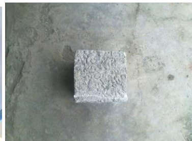
Fig.9 View of Specimen after Acid resistance Test
